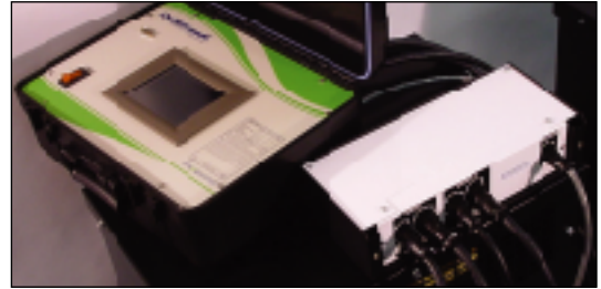
SIMPLE TWISTLOCK CONNECTION TO POWERSMITHS SMART1 INTEGRATED TRANSFORMER METERING PORT
